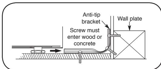
The Anti-tip bracket is packaged with an installation template.
