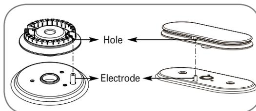
Make sure the hole in the burner head is positioned over the electrode.
